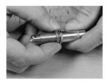
**4.** While holding the endpin jack from the inside of the guitar, install the smaller dress washer followed by the smaller hex nut on the outside where the jack is protruding from the guitar.
