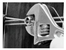
**6.** Install the strap button and tighten with pliers using rubber or leather to protect the strap button.
