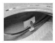
8. Using a Phillips head screwdriver, loosen the cork padded mounting clamps on each side until the clamps are fully open and insert the pickup into the soundhole. You want the pickup to be as close to the neck as possible. Tighten the clamps gently until the pickup is secure. String the guitar and adjust the pickup as needed centering the logo under the strings.
