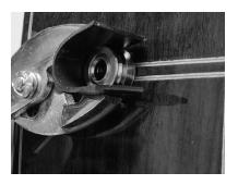
7. Install the 2 self-adhesive wire clips to the inside of the guitar and hook the pickup lead wire into the bendable tabs securely out of the way. Preferably on the inside waist of the guitar.
