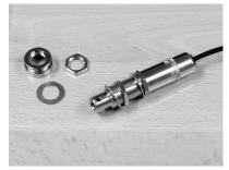
3. Adjust the length of the larger threaded barrel by moving the large hex nut along with the dress washer and star washer until the smaller portion of the threaded barrel fully extends through the tailblock. It should extend no more than 11/32" (8.7mm) or a minimum of 5/16" (7.9mm) outside of the guitar.
