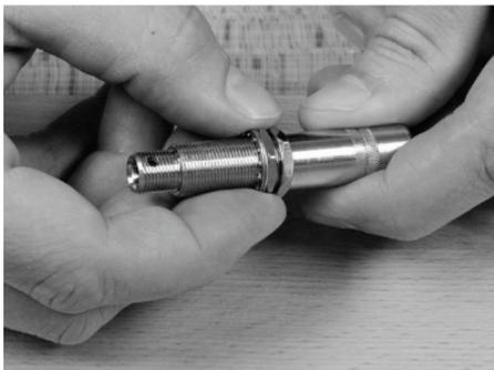
4. While holding the endpin jack from the inside of the guitar, install the smaller dress washer followed by the smaller hex nut on the outside where the jack is protruding from the guitar.
