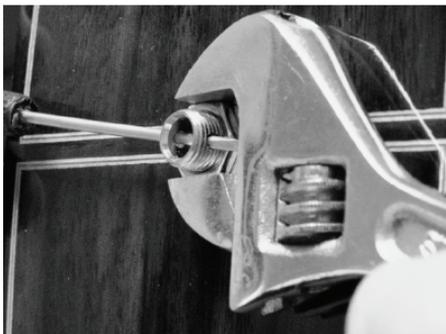
6. Install the strap button and tighten with pliers using rubber or leather to protect the strap button.
