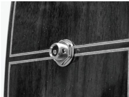
5. Using a small screwdriver or hex wrench through the hole of the endpin jack, hold the jack in place while tightening the hex nut with an open end 1/2" wrench or adjustable pliers.
