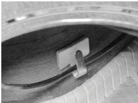
8. Using a Phillips head screwdriver, loosen the cork padded mounting clamps on each side until the clamps are fully open and insert the pickup into the soundhole. You want the pickup to be as close to the neck as possible. Tighten the clamps gently until the pickup is secure. String the guitar and adjust the pickup as needed centering the logo under the strings.
